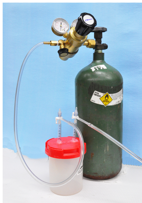
Figure 1. Closed container system with valve used to maintain hyperoxic gas environment. Plates were placed in a 1 L airtight container. Air was removed using a vacuum tube connected to a standard laboratory vacuum gas tap. Pure oxygen was inserted via a PVC tube connected to a compressed gas cylinder and the container was incubated at 37°C.
