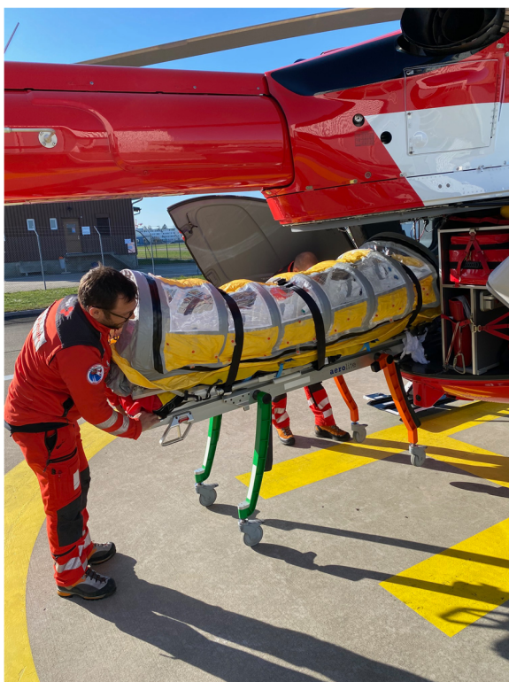
Fig. 2 Rega PIU HEMS: Loading or unloading of the patient in the PIU
