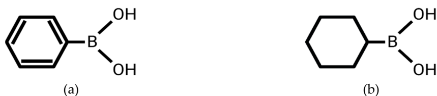
Figure 1. A schematic representation of the molecular structure of (a) phenyl boronic acid (PBA) and (b) cyclohexyl boronic acid (CHBA).
