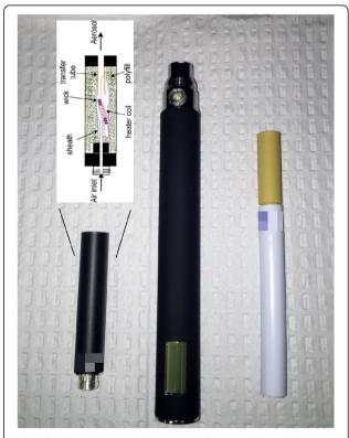
**Fig. 1** Study products with cartomizer schematic. The cartomizer, battery, and cigarette substitute are shown here (L to R). There is also a schematic of the cartomizer generously provided by Dr. Alan Shihadeh
