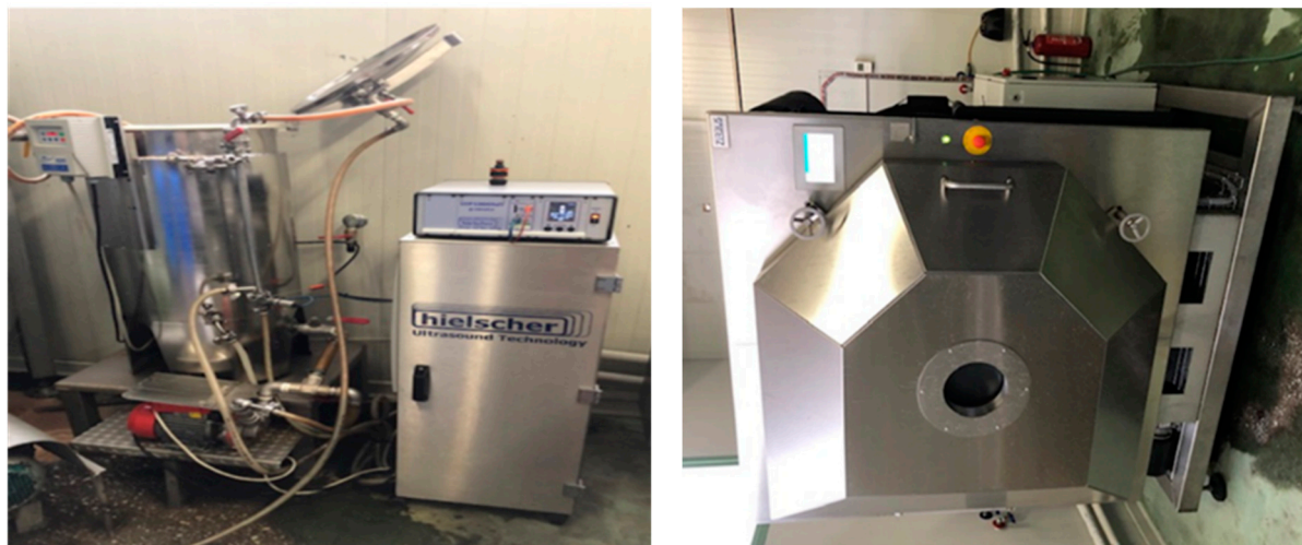
Figure 5. Industrial ultrasound homogenizer, Hielscher model UIP1000hdT (left) and industrial freeze dryer Zirbus GmbH model EKS 100-109 (right).
