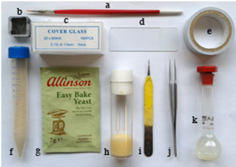
Figure 1. Required materials: a. fine pen brush, b. small square broken-glasses container, c. 22 x 50 mm coverslip, d. microscope slide, e. double-sided sticky tape, f. dry yeast powder in test tube with holes on the lid, g. yeast granule used for fly maintenance, h. fly food vial, i. a half of a tweezers used for dechorionate embryos, j. a pair tweezers, k. heptane glue liquid container (volumetric flask).
