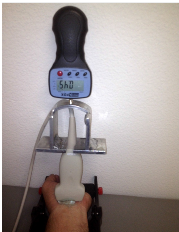
Figure 1. The device developed to apply pressure to the wrist and hand consisted of an algometer in series with an ultrasound imaging probe. By pressure being applied through the algometer, the pressure under the ultrasound probe could be measured and correlated to changes in the internal structures in the hand.
