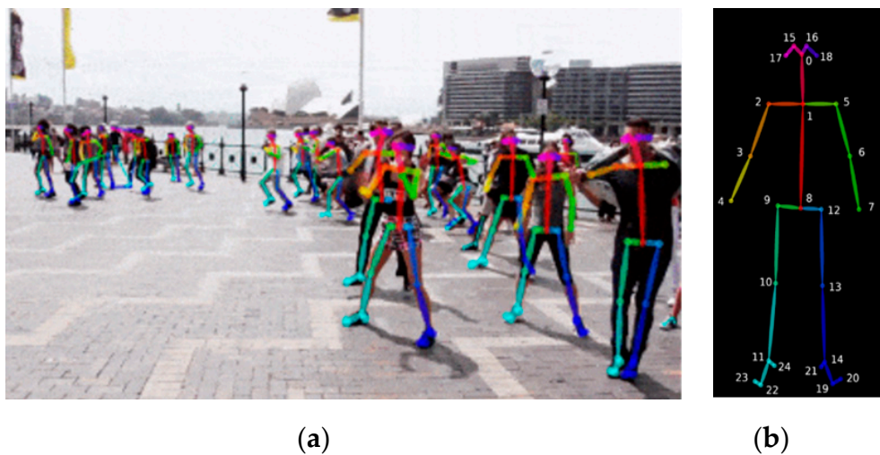
Figure 1. Skeleton extraction based on OpenPose: (a) Multi-person skeleton extraction; (b) Diagram of the human skeleton key points.
