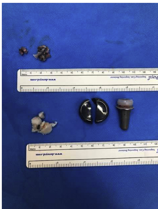
Figure 2 Intraoperative pictures showing the fractured pyrocarbon head, concomitant capitellar chondral shear injury, and carbonised synovium with pyrocarbon particles.
