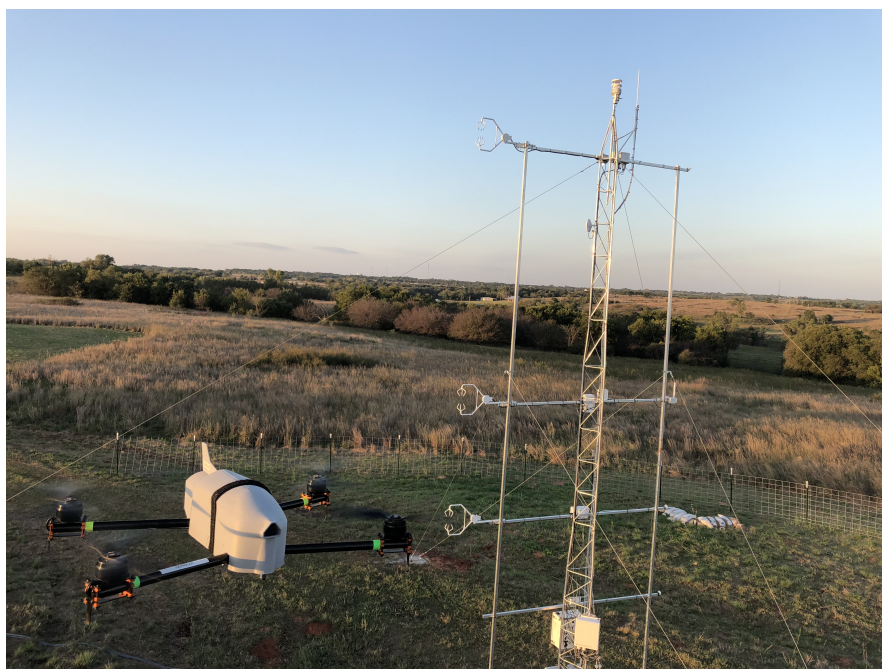
Figure 6. Picture showing the CopterSonde in flight near a meteorological tower.
