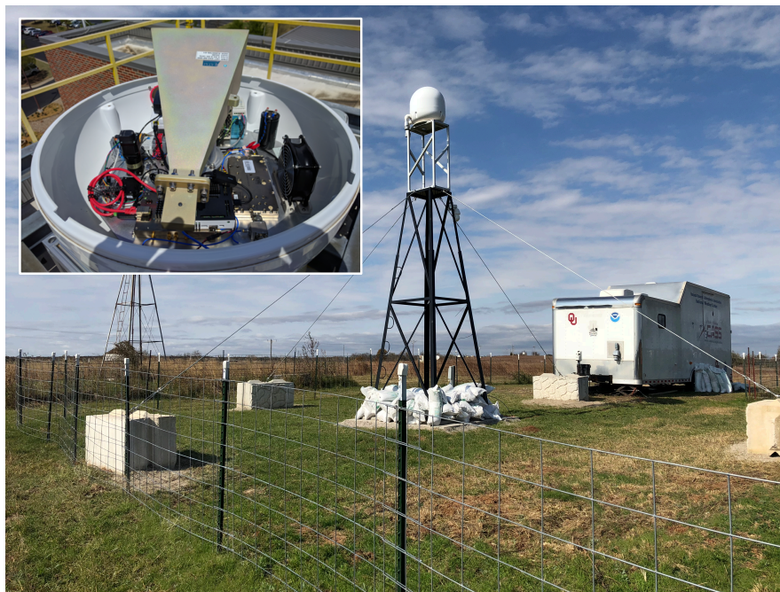
Figure 8. Picture of the GeoFence Radar mounted on a tower at KAEFS with an inset picture showing the radar hardware.
