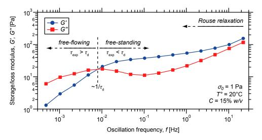
**Figure 6.** Oscillatory frequency sweep on a metallo-supramolecular hydrogel prepared from P(DMAMEA<sub>200</sub>-*co*-TpyMA<sub>4.5</sub>) copolymer and 0.5 eq of Co (II) ions.
