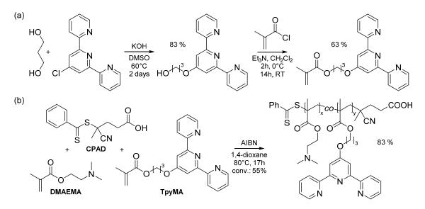
**Figure 2.** (a) Synthesis of terpyridine-functionalized methacrylate monomer; (b) Synthesis of side-chain terpyridine-functionalized poly(2-(dimethylamino)ethyl methacrylate).
