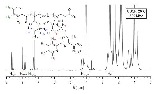
**Figure 3.** <sup>1</sup>H NMR spectrum of pure P(DMAMEA<sub>200</sub>-*co*-TpyMA<sub>4.5</sub>) copolymer in deuterated chloroform as solvent.
