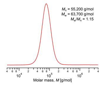
**Figure 4.** Size exclusion chromatrography (SEC) traces for of pure P(DMAMEA<sub>200</sub>-*co*-TpyMA<sub>4.5</sub>) copolymer (molar masses are given with respect to polystyrene standards).
