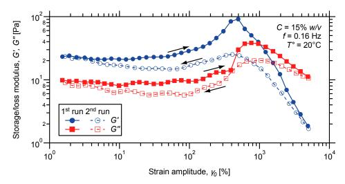
**Figure 7.** Oscillatory strain sweeps (arrows indicate up and down sweeps) on a metallo-supramolecular hydrogel prepared from P(DMAMEA<sub>200</sub>-*co*-TpyMA<sub>4.5</sub>) copolymer and 0.5 eq of Co (II) ions.
