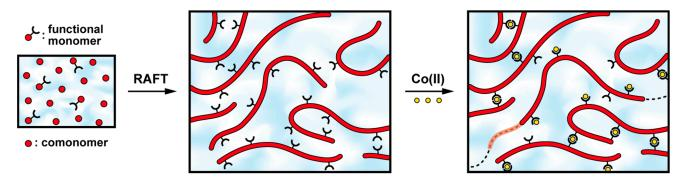
**Figure 1.** Schematic representation for the synthesis of a side-chain ligand-functionalized copolymer and its assembly into a metallo-supramolecular gel.
