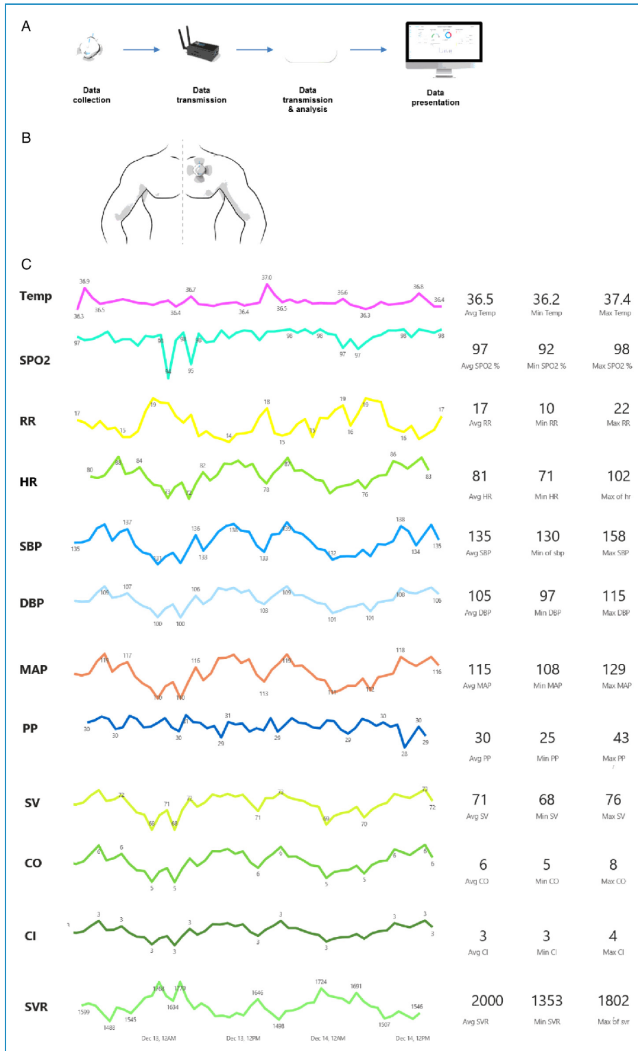
Figure 1. The remote patient monitoring system used in the study. (A) The architecture of the wearable monitoring system; (B) a figure showing the device and its positioning on a patient’s chest; (C) a monitoring sample of the photoplethysmography-based device with mean values in a single patient.
