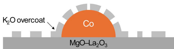
Scheme 1 Schematic illustration of the proposed surface structures of the K-Co1 catalysts.
