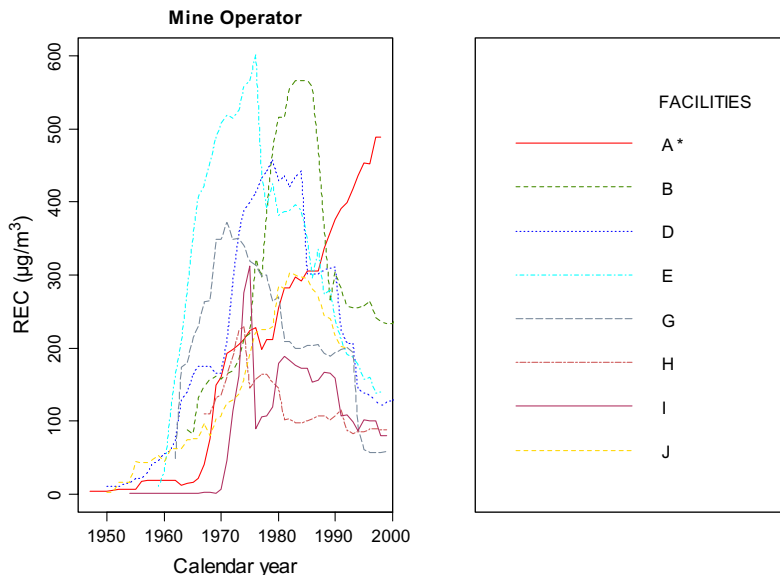
Fig. 3. REC historical predictions ( \mu\text{g}/\text{m}^3 ) for the mine operator are shown, based on the primary facility-specific CO models, by mining facility. Footnote (*) Facility A had no mine operator and therefore the loader operator is depicted.
