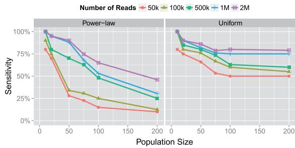
Fig. 5. Assembly accuracy estimation. Up to 200 viral genomes were generated from the Gag/Pol 3.4 kb HIV region. The population diversity is 3–20%. Viral genome abundances follow power-law and uniform distributions. Consensus error-corrected 2100 bp paired-end reads were simulated from HIV population
