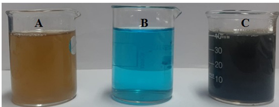
Figure 2. The colour changes from pale yellow to dark colour of Wt -CuNPs a) \text{CuSO}_4 solution b) Wrightia tinctoria R.Br c) Synthesized Wt -CuNPs.
