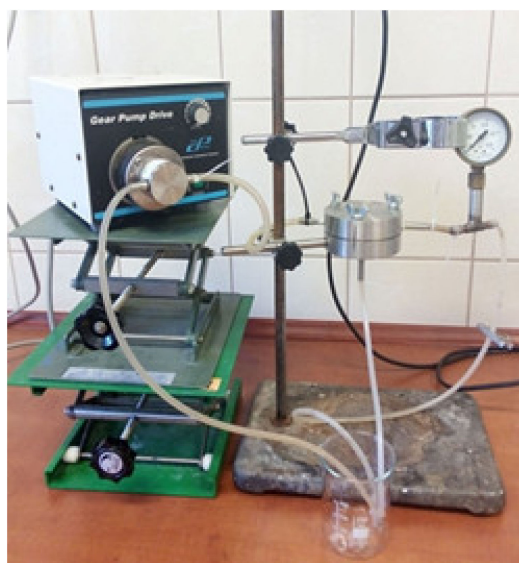
Figure A1. The laboratory filtration unit: Gear pump (Cole Parmer, Vernon Hills, IL, USA), steel module for membrane, and monometer. Pressure is generated by throttling.
