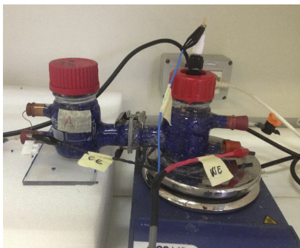
Fig. 2. Experimental BES-Pot, gravel test setup.
