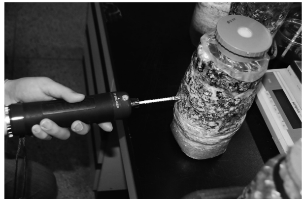
Fig. 3. Measurement of CO 2 (%) in a 1.3 kg Lentinula edodes cultivation sawdust bag using a gas sampler (Model GV-110S; Gasteko, Ayase, Japan) and CO 2 core sword (2H, 2HH; Gasteko).
