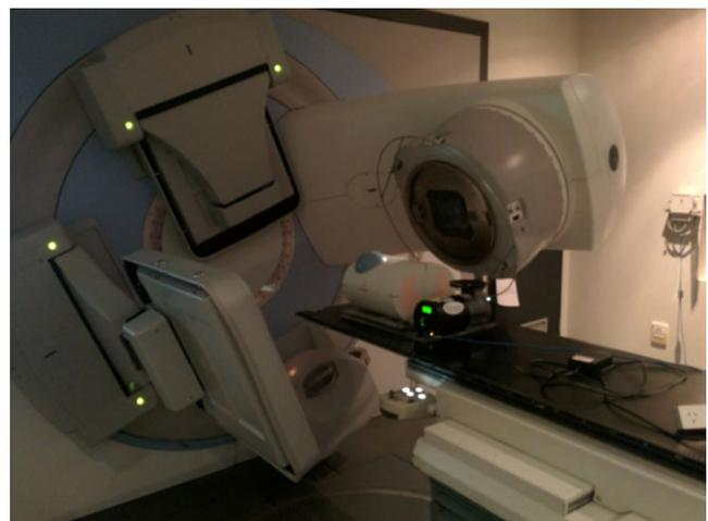
**FIG. 1.** The experimental setup for simulating the effects of motion on breast radiotherapy. The direction of one-dimensional motion was along the longitudinal couch direction.
