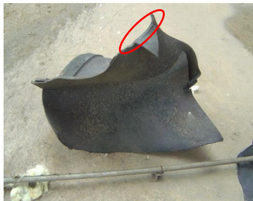
Figure 10. The photo of the cracked blade in the A fan.
