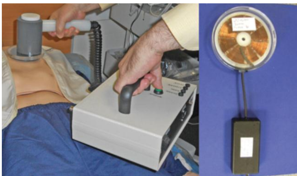
Figure 2. Prototype hand-held ( ex vivo ) radio frequency (RF) power-transmitter and prototype battery-free implantable ( in vivo ) power-receiver (encapsulated for bench characterisation).
