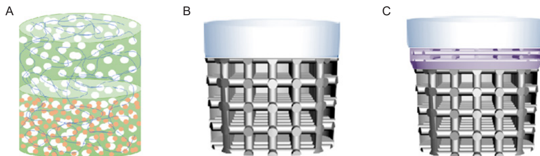
Figure 1. Scaffolds intended for osteochondral regeneration developed in Biomaterials and Additive Manufacturing: Osteochondral Scaffold (BAMOS) project and tested in vivo . (A) Enzymatically cross-linked silk fibroin-based bilayered scaffold. (B) Titanium-collagen/poly(lactic-co-glycolic acid) bilayered scaffold. (C) Titanium-poly(lactic acid)-collagen/poly(lactic-co-glycolic acid) trilayered scaffold.
