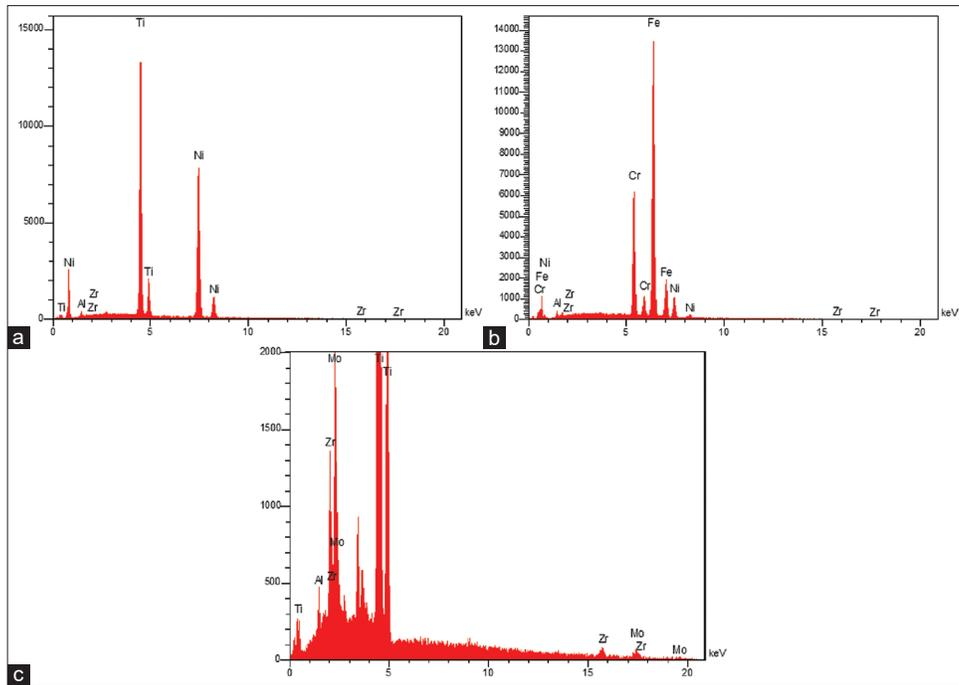
Figure 4: EDX (a) NiTi with coating, (b) SS with coating, and (c) TMA with coating
