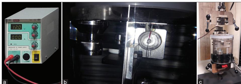
**Figure 1.:** (a) Transformer applying 12 v voltage; (b) fixture; (c) designed device to be positioned on the lower compartment of the universal testing machine
