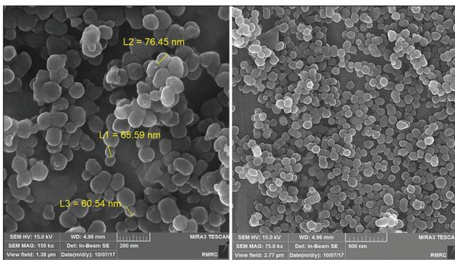
Figure 5: FESEM images of TMA coated wire at 200 and 500 nm magnifications
