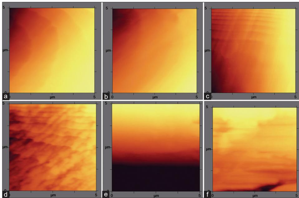
**Figure 2:** TopoFwd images (a) NiTi, (b) NiTi with coating, (c) SS, (d) SS with coating, (e) TMA, (f) TMA with coating
