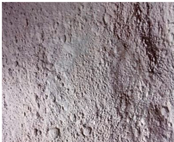
Fig. 1. Admixture of MK and BLA powder (BLA + MK).
