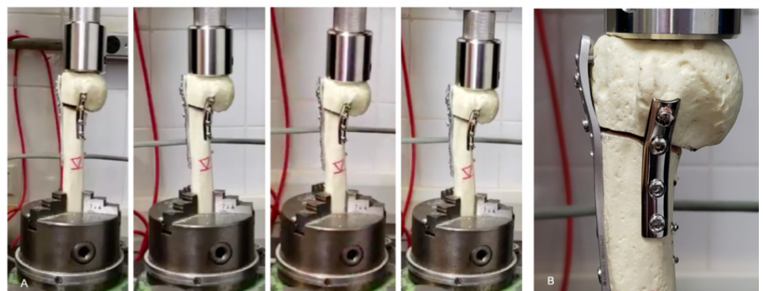
Fig 4. Sequence of mechanical testing in one model of Group L+T. A. Four phases identified during the test. Note that gradually humerus head suffered substantial varus collapse and both medial and lateral gap disappear; B. Mode of failure of Group L+T: there were obvious loosening of the proximal part of the lateral locking plate from the humerus head due to varus displacement. In addition, the two most proximal screws from the anteromedial nonlocking plate pushed out from the humerus head as well. There were no signs of breakage of any screws or plates nor hardware cut-out or cut-through.
