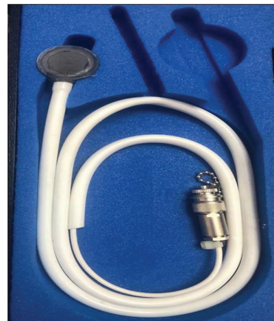
Figure 2: Parallel plate ionization chamber (PRATT2)
