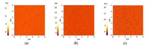
**Figure 3.** Atomic Force Microscopy (AFM) images of magnetron sputtered PTFE-like thin films deposited for 30 min at various RF powers: (**a**) 50 W; (**b**) 80 W; and (**c**) 110 W.
