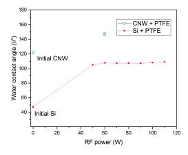
**Figure 13.** The dependence of the water contact angle on applied RF power for the PTFE-like magnetron-sputtered thin films.
