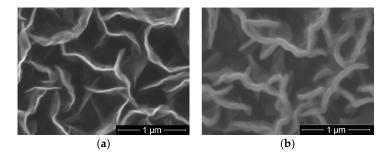
**Figure 5.** SEM images of carbon nanowalls (CNW) (**a**) as-deposited; and (**b**) covered by PTFE layer deposited by magnetron sputtering.
