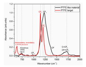
**Figure 2.** Fourier Transform Infrared (FTIR) spectra of the PTFE target (**red curve**) and PTFE-like material obtained by radiofrequency (RF) magnetron sputtering (**black curve**).
