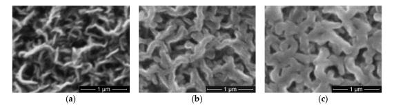
Figure 8. SEM images of CNW treated with C<sub>2</sub>H<sub>2</sub>F<sub>4</sub> plasma for (a) 2 sccm; (b) 8 sccm; and (c) 36 sccm.
