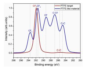
**Figure 1.** High-resolution spectra of C1s region for PTFE target (**red line**) and magnetron-sputtered PTFE material (**blue line**).
