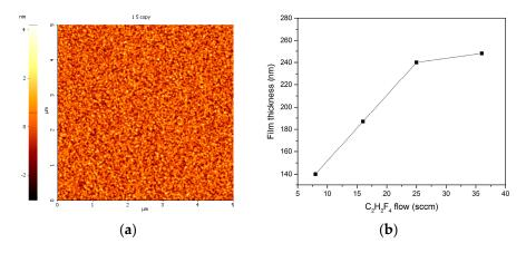
**Figure 7.** (a) Typical topography of fluorocarbon film deposited on flat Si substrate by plasma assisted chemical vapor deposition (PACVD) of  $C_2H_2F_4$  (25 sccm flow); and (b) dependence of deposition rate on  $C_2H_2F_4$  flow rates.
