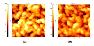
**Figure 9.** The topography of CNW after fluorocarbon plasma exposure with (**a**) 8 sccm (Root Mean Square (RMS) 69.7 nm); and (**b**) 16 sccm (RMS 80.2 nm) of  $C_2H_2F_4$ .
