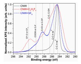
Figure 6. Normalized high-resolution spectra of CNW and treated CNW by  $SF_6$  and  $C_2H_2F_4$  plasma.
