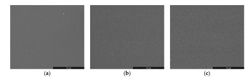
**Figure 4.** Top view Scanning Electron Microscopy (SEM) images of the magnetron sputtered PTFE materials upon injected RF power to the plasma source: (**a**) 50 W; (**b**) 80 W; and (**c**) 110 W.
