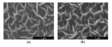
Figure 10. SEM images of CNW treated with SF<sub>6</sub> plasma for (a) 8 sccm; and (b) 36 sccm.
