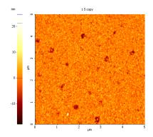
Figure 12. Surface topography of Si after 36 sccm SF<sub>6</sub> plasma treatment.
