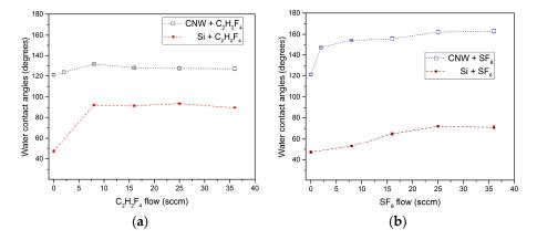
**Figure 14.** Contact angles of CNW layers and Si wafer after plasma exposure to (**a**)  $C_2H_2F_4$  PACVD process; and (**b**) SF<sub>6</sub> plasma treatment.
