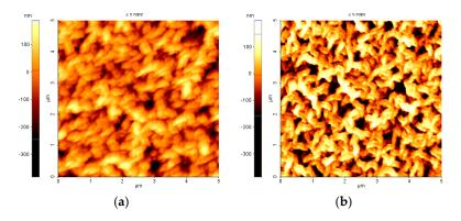
Figure 11. The topography of CNW after SF<sub>6</sub> plasma treatment using (a) 2 sccm; and (b) 36 sccm.
