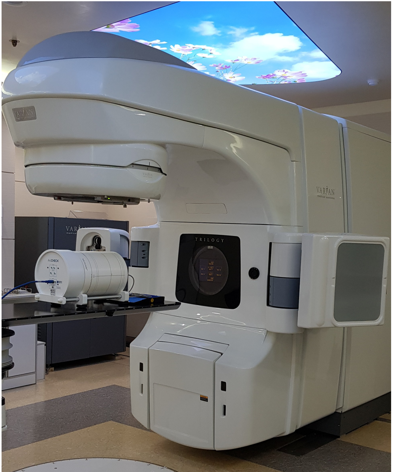
Fig 5. Dose measurement with ArcCHECK for the dose reconstruction with the 3DVH program.
