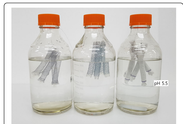
Fig. 3 An experimental duodenal pH environmental model. Distilled water at pH 5.5 was put in the reservoirs, and 5 antireflux stents of each type were placed so that the distal part could be submerged
