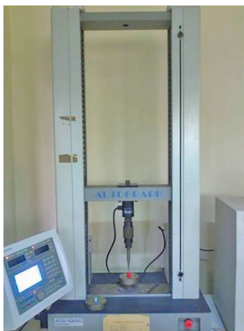
Fig. 4: Measuring fracture strength by universal testing machine
