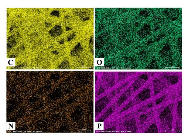
Figure 2. SEM mapping results of ACF-10.3% PDPP.
