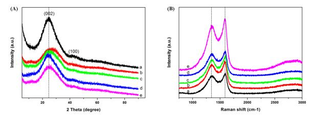
**Figure 3.** (**A**) XRD patterns and (**B**) Raman spectra of (**a**) ACF-0; (**b**) ACF-3.9% PDPP; (**c**) ACF-6.4% PDPP; (**d**) ACF-10.3% PDPP; and (**e**) ACF-12.9% PDPP.
