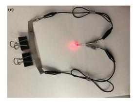
**Figure 7.** Electrochemical performance of ACF-10.3% PDPP-based symmetric supercapacitor: (a) long-term cycle stability test at a current density of  $10 \text{ A} \cdot \text{g}^{-1}$ ; (b) CV curves of ACF-10.3% PDPP bended by different angles (0°, 90° and 180°) at a scan rate of 100 mV·s<sup>-1</sup>; and (c) digital photo images of a red LED powered by three devices in series.
