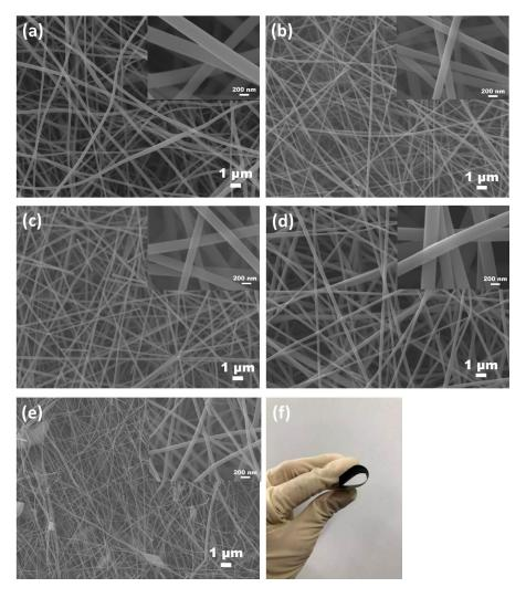
Figure 1. SEM images of (a) ACF-0; (b) ACF-3.9% PDPP; (c) ACF-6.4% PDPP; (d) ACF-10.3% PDPP; (e) ACF-12.9% PDPP; and (f) optical image of ACF-10.3% PDPP.
