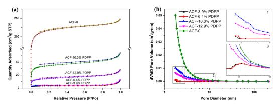
**Figure 5.** (a) Nitrogen adsorption and desorption isotherms, and (b) pore size distribution of ACF-0, ACF-3.9% PDPP, ACF-6.4% PDPP, ACF-10.3% PDPP, and ACF-12.9% PDPP samples.
