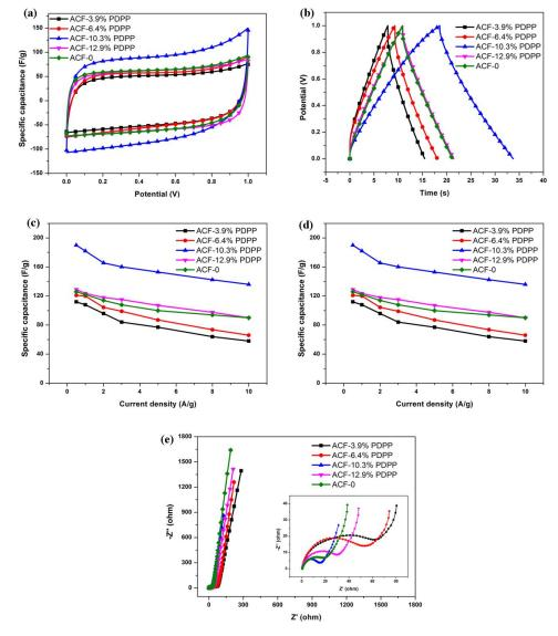
**Figure 6.** (a) CV curves of all samples at a scan rate of 30 mV·s<sup>-1</sup>; (b) GCD curves of all samples at current densities of 5 A·g<sup>-1</sup>; (c) specific capacitance of each sample at different current densities (0.5–10 A·g<sup>-1</sup>); (d) Ragone plots as a function of current densities (0.5–10 A·g<sup>-1</sup>) of symmetric supercapacitors; and (e) Nyquist plots of all samples in the frequency range of 100 kHz and 0.01 Hz. The inset in (e) is the magnified region.
