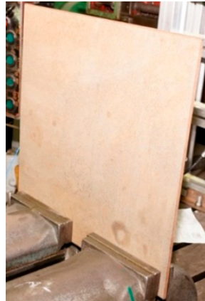
Figure 4. P1 plate (without welded joints) mounted on a test bench.
