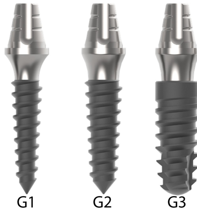
Fig 1. Representative image of the implants tested in each group. The groups G1 and G2 are one-piece implants and the group G3 is two-pieces implant.
