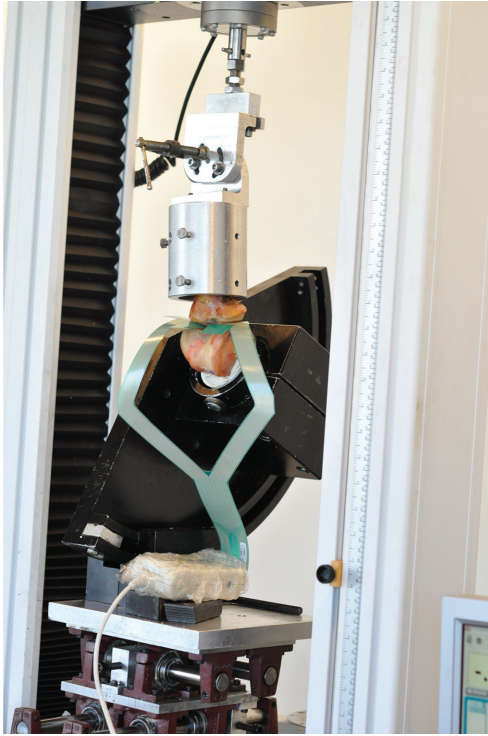
Figure 1. Knee specimen mounted on an Instron materials testing system at 30° of flexion.
