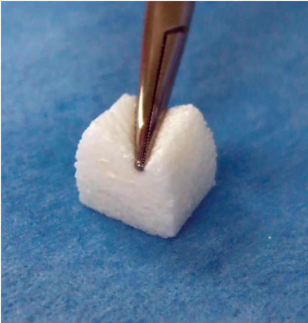
Fig. 1. Bioabsorbable artificial bone. This is an HA/Col composite (RIFIT, HOYA Co Ltd, Tokyo, Japan) with a bone-like nanostructure, 35% porosity, and a 100- to 500- \mu m pore diameter.
