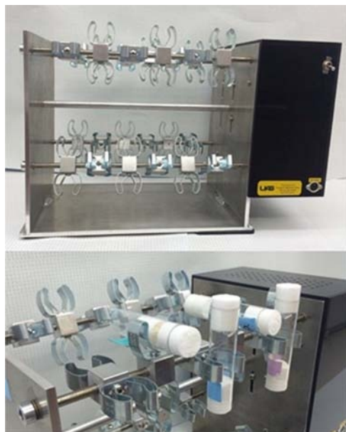
Figure 3. The TreadWheel provides a low-impact exercise stimulus for Drosophila . Rotating arms induce continuous walking in several Drosophila vials simultaneously. Unexercised cohorts have foam stoppers inserted close together to restrict movement and control for machine exposure, visible in close-up photo (below).
