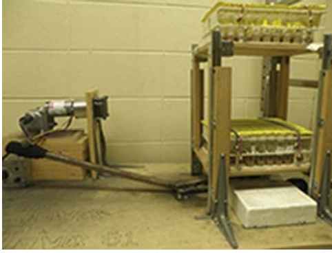
Figure 1. The Power Tower, a motor-operated enforced climbing apparatus that exercise trains Drosophila . As the rotating arm circles around in a clockwise direction, the lever pushes down and the two platforms of vial holders rise up. As the rotating arm rolls off, the lever lifts and the platform of vial holders drops down. The flies drop to the bottom of the vial, inducing their negative geotaxis instinct. The flies continue to repeat this process until the motor is shut off. Exercise training thus occurs through continuous climbing.
