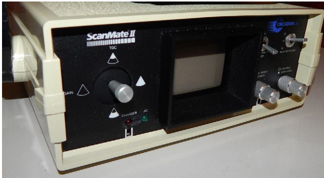
FIGURE 1 Controls for the ScanMate II ultrasound machine included: a toggle knob for the time gain compensation; 3 depth settings at 10, 14, and 18 cm; power on/off switch; and adjustments for scan angle, contrast, and brightness
