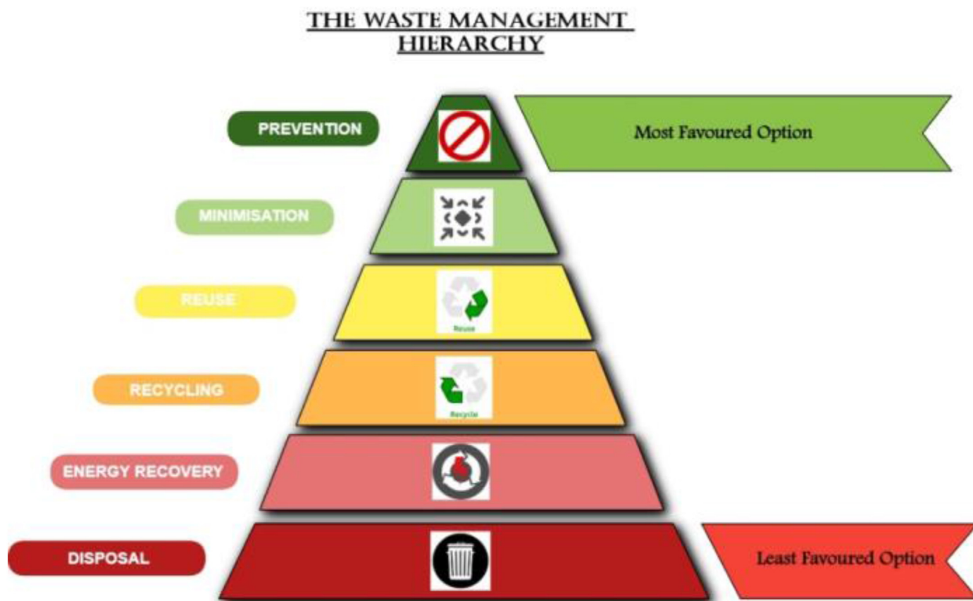
Figure 6. Triangular diagram of Waste Management Hierarchy. The order of preference for waste reduction and effective management are illustrated in the upward triangular diagram.
