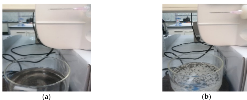
Figure 1. Dripping of 1% ALG solution (a) and ALG–BPA (1:1) (b) in a CaCl_2 bath.
