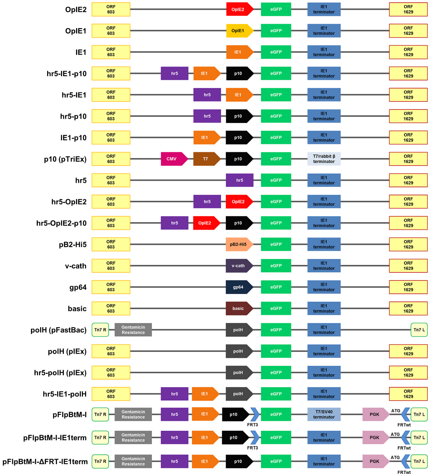
Fig 1. Schematic overview presenting all expression vectors used in this study. This overview describes the genetic elements of all expression vectors used in this study. The ORF603 and ORF1629 are essential recombination elements required for the flashBAC system [9,50]. Tn7 R/L and the gentamicin resistance are required for the Bac-to-Bac system (Life Technologies). Terminator sequences are shown in blue boxes, eGFP as model protein in green. The long arrow-like symbols indicate promoter regions. hr5 is a homologous region and functions as an enhancer. The blue short arrow-like symbols represent
