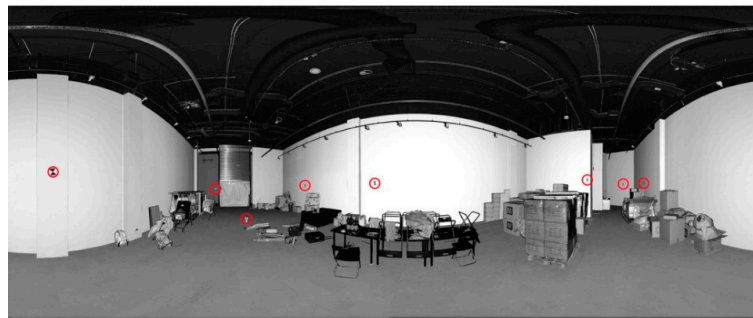
Figure 6. An example of the point cloud in the spherical projection of Test Site IV: “Empty Shop (shopping mall)” with marked check points (red circles) [27].
