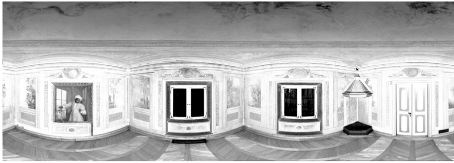
Figure 3. The point cloud in the spherical projection of Test Site II: “The Chamber with a Parrot” without marked points [27].
