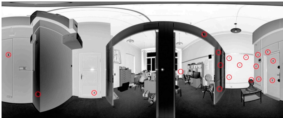
Figure 4. An example of the point cloud in the spherical projection of Test Site III: “The Office” with marked check points (red circles) [27].
