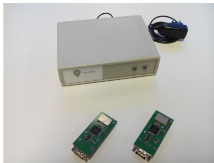
Figure 1. Evaluation module of the implemented Social Sensor device and a Home Hub.
