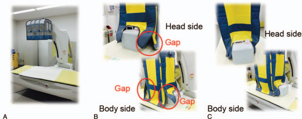
Figure 4. Measurement conditions. Measurements were performed without the additional lead shielding device (A), with the additional lead shielding device and with a gap in shielding (B), and with the additional lead shielding device and without a gap in shielding (C). The upper part of the device is made of mesh.
