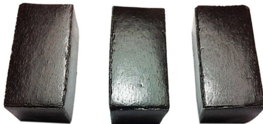
Figure 3. Specimens for the compressive strength test.
