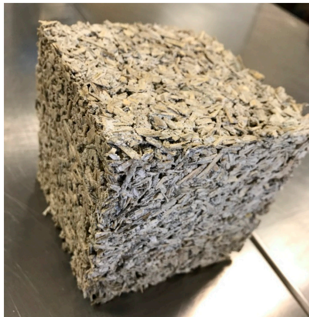
Figure 1. Hemp–lime composite mixture 1.
