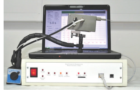
FIGURE 1: The surgical robot drilling system used in cochleostomy supported on a fixed flexilock arm.
