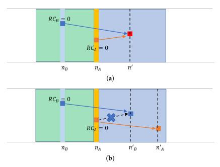
**Figure 2.** Use of the lookahead. (a) SPS cannot resolve the collision if two close UEs choose the same resource. (b) SPS/LA can resolve most potential collisions; *A* knows *B*'s planned movement through the received lookahead in *B*'s packet
