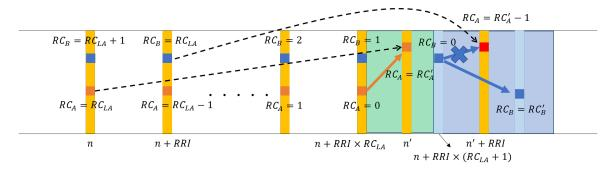
Figure 3. SPS sensing prevents the collision of the planned moves if RCs expire in different subframes.
