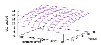
**Figure 5.** Number of additional bits to include the lookahead in the SCI Format 1, including the ten offset bits to the subframe in the lookahead.
