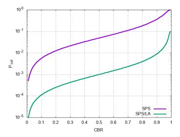
Figure 6. Collision probabilities upon reselection under SPS and SPS/LA.
