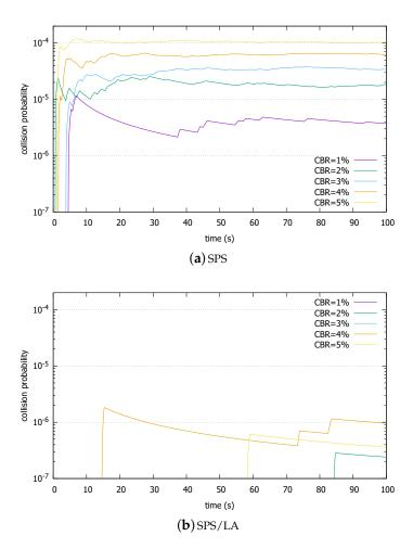
Figure 7. Packet collision rates comparison in (a) SPS and (b) SPS/LA, light load.
