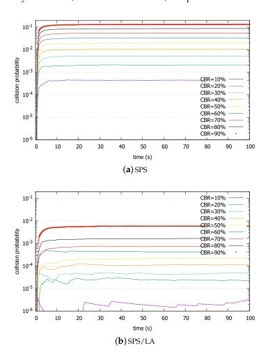
Figure 8. Packet collision rates comparison in (a) SPS and (b) SPS/LA, heavy load.
