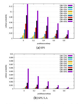
Figure 10. Collision probabilities under varying probResourceKeep, heavy load. (a) SPS. (b) SPS/LA.
