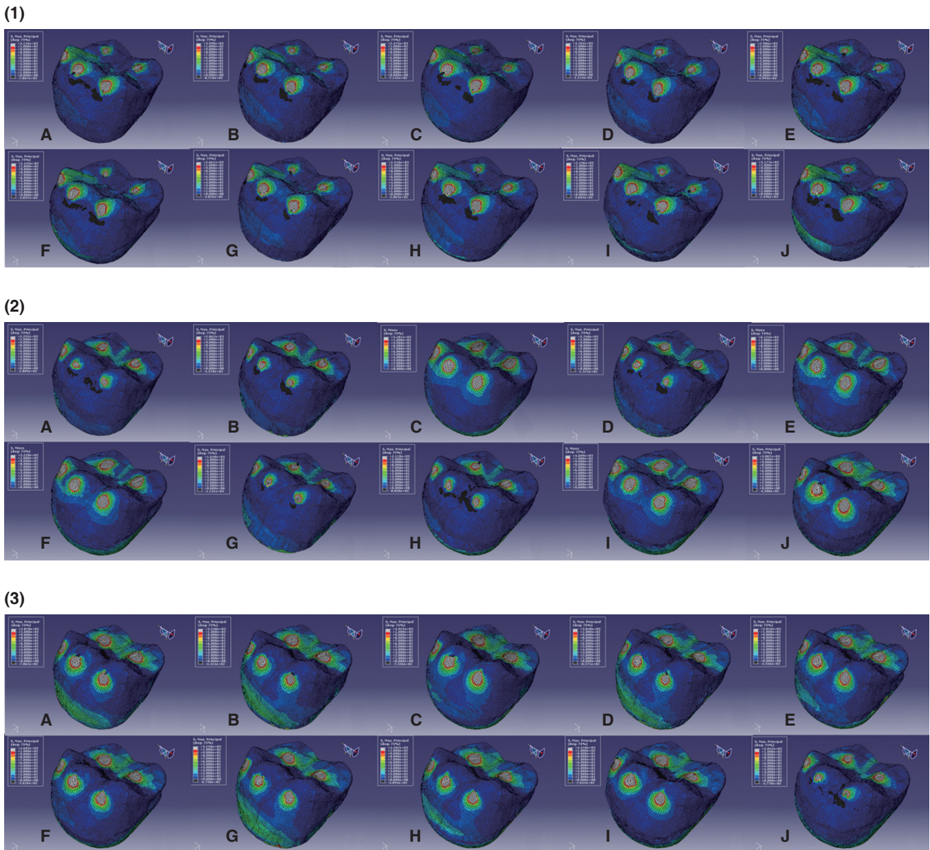
Fig. 6. Maximum principal stress distributions of 10 models subjected to masticatory force (under the application of loads from three directions). (1) load of 280 N at 0° to the tooth axis (vertical direction), (2) load of 280 N at 45° to the tooth axis, towards the lingual margin, and (3) load of 280 N at 90° to the tooth axis, towards the lingual surface (horizontal direction). A: Model 1, B: Model 2, C: Model 3, D: Model 4, E: Model 5, F: Model 6, G: Model 7, H: Model 8, I: Model 9 and J: Model 10.
