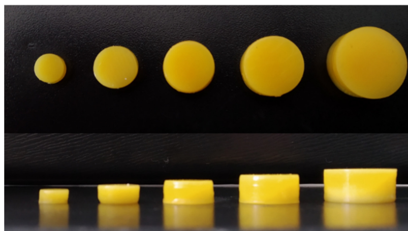
Figure 12. Top and side views of 3D printed MEB-loaded tablets with different volumes.
