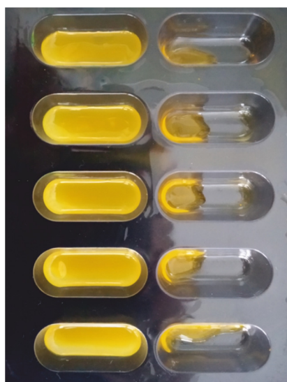
Figure 2. Examples of cured (left side) and uncured (right side) resins in blisters after 30 min of exposure to visible light and rinsing out the residual resin.
